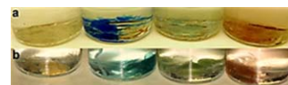
Figure 7. Color changes of heavy metal aqueous solutions of a) MBAGD-A and b) MBAMP-A upon hydrogel adsorption. From left to right: Native resins, \text{Cu}^{2+} , \text{Ni}^{2+} , and \text{Co}^{2+} solutions. [Color figure can be viewed in the online issue, which is available at wileyonlinelibrary.com .]
